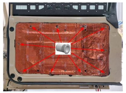
Drill out the door panel mounting holes to 9mm and fasten the M6 Riv-Nuts into the holes M6 Rivnut
