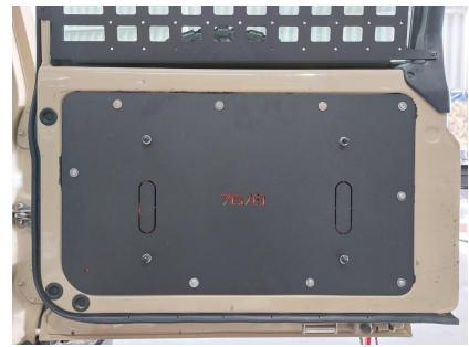
Place the M6 cage nuts into the 4 x square holes in the mounting plate, from the back side of the plate.
