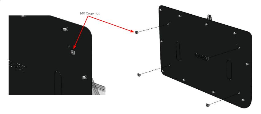
Fasten the Drop-Down Table to the mounting plate throught the slotted holes on the Drop-down Table using the M6 Button-head bolts, the spring washers and the flat washers which thread into the cage nuts in the mounting plate.
