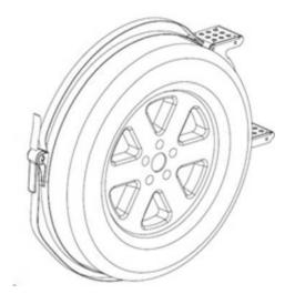
Place the steps over spare wheel and thread the end of strap through ratchet.
